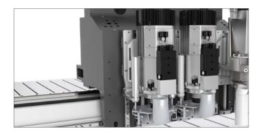
Choose a single, double or even triple-head configuration for applications that typically require multi-tool cutting operations. A twin carriage option is also available, enabliing you to copy cut two parts at the same time, effectively doubling production capacity and enabling a faster turnaround on jobs.
