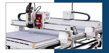
Dual gantries on a single machine deck offer a compact and cost-efficient alternative to purchasing two router tables. The independently driven gantries allow simultaneous processing of the same or different jobs even with different tools on both ends of the table.
