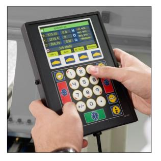
The AXYZ SmartConsole brings unprecedented ease of use, context sensitive menus, real-time display of machine status and many more time-saving, functional and productivity features. It provides a graphical preview and current status of a running job and allows program feeds and speeds to be changed without pausing the program.
