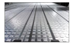
The innovative design of the aluminum vacuum deck allows zoned areas to be opened or closed as needed. Flat sheet materials are held as securely as possible while cutting problems caused by movement or vibration of the materials are virtually eliminated.
