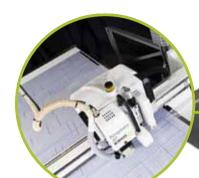
*i*-cut Vision Pro: The Kongsberg XN can be controlled by *i*-cut Vision Pro, the industry standard for vision-based cutting. It ensures highly efficient production along with simple and extremely accurate print-to-cut registration, even with print-distorted materials.
