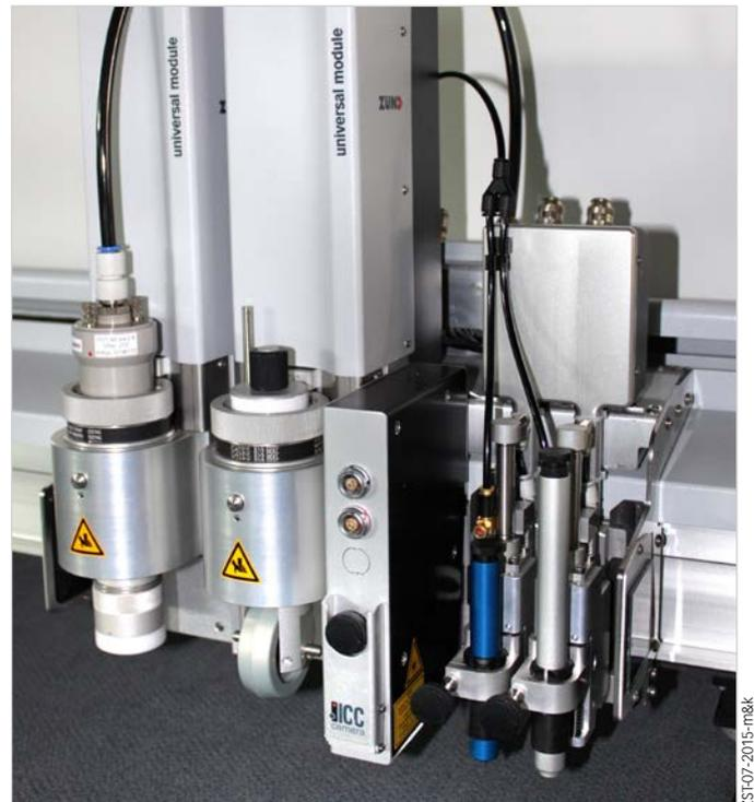
Fully equipped module carrier with 2 UM, ICC Camera and MAM-D.
